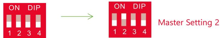
4. If the battery communicates with the Growatt SPF HVM-P/ES/WPV by RS485 communication, turn the master DIP switch "#2" and "#3" to "ON".
