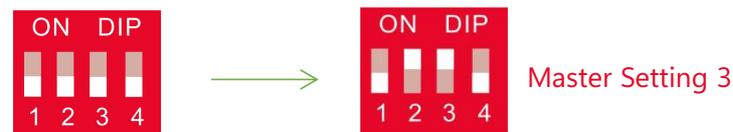
5. If the battery communicates with the Schneider Conext Series, turn the master DIP switch "#1" and "#3" to "ON".
