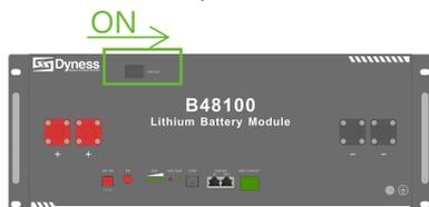
2. Press SW button 3s to wake up battery
