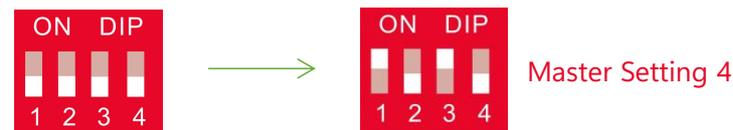
6. When you setup the master DIP as setting 1~4, all the slaves keep the DIP 0000, no need change.
