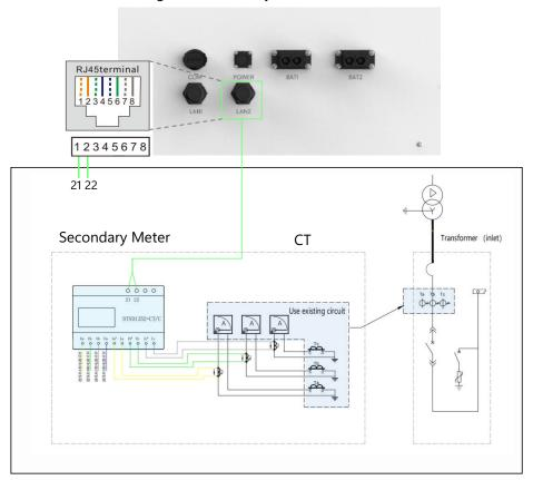
Figure 5-15 Secondary meter installation
