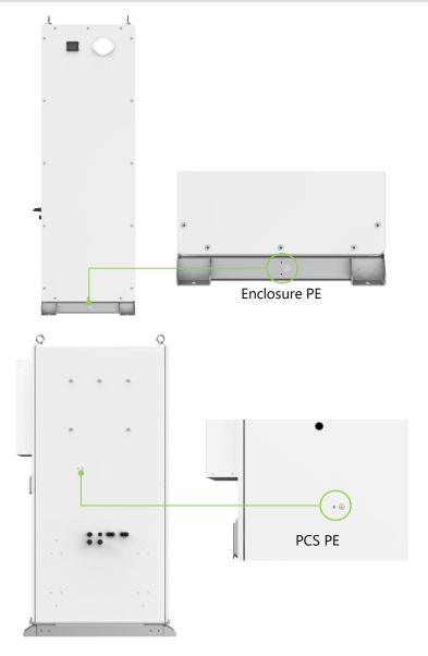
Figure 5-10 Battery Grounding
