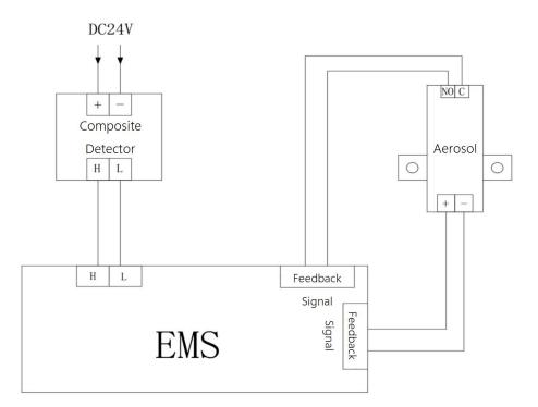
Figure 3-7 Fire Protection principle
