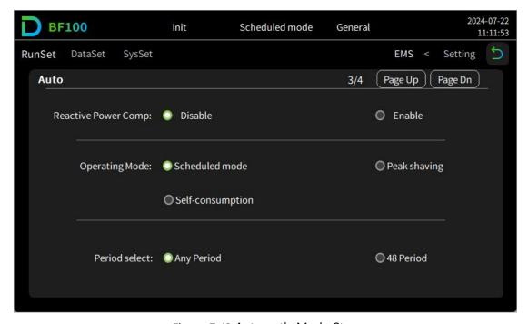
Figure 7-13 Automatic Mode Step
