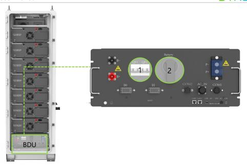
Figure 5-9 Breakers Location
