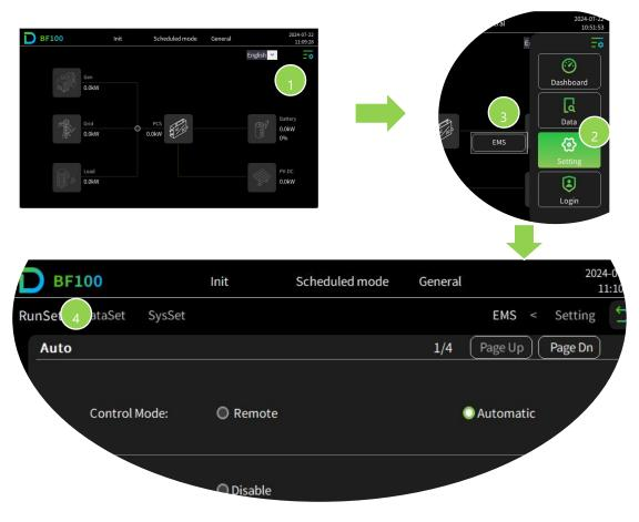
Figure 7-7 Running Setting Step
