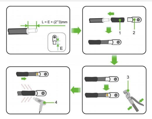
Figure 5-8 The Connection Sequence of Wiring Components
