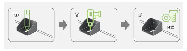
Figure 5-4 Angle Iron Brackets Installation Steps
