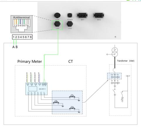
Figure 5-14 Primary meter installation
