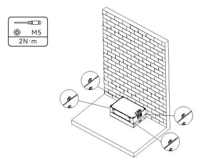
Step 4: Repeat steps 2 and 3 until the required batteries and BDU are installed.
