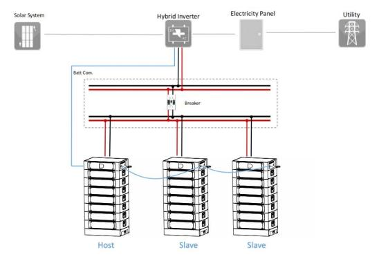
Figure 5-1 The general configuration diagram of the STACK100
