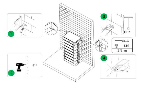
1. Mark the hole positions using a marker.
