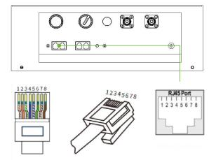
Figure 2-12 "Inverter CAN/RS485" port pins
