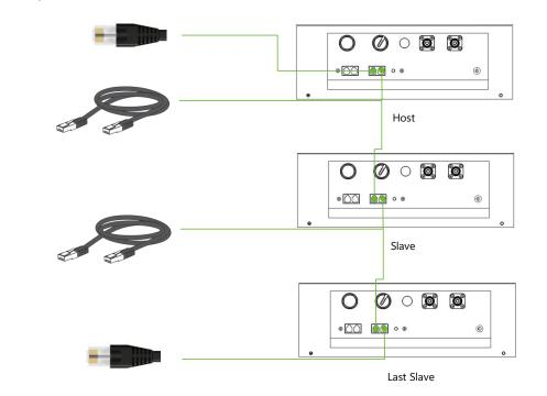
Communication network cable connection between inverter and STACK100(Host): CAN/RS485 of the BDU of STACK100 to the communication port of the inverter.
