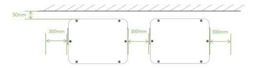
Figure 3-1 The Minimum Clearance Diagram
