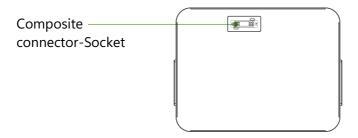
Figure 2-4 HV9637 Bottom Interface
