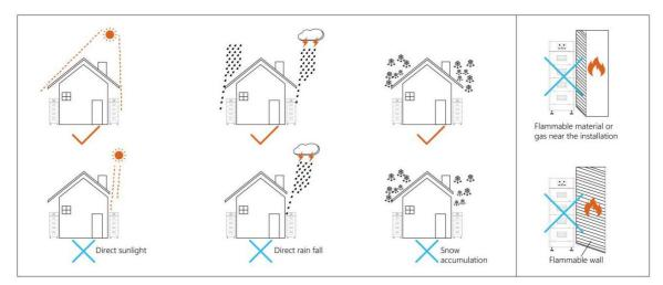
Figure 3-2 Installation Location Precautions
