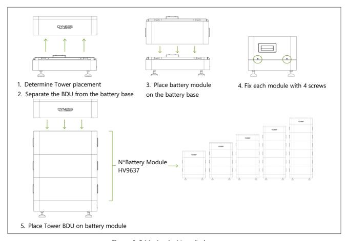
Figure 3-5 Mechanical Installation
